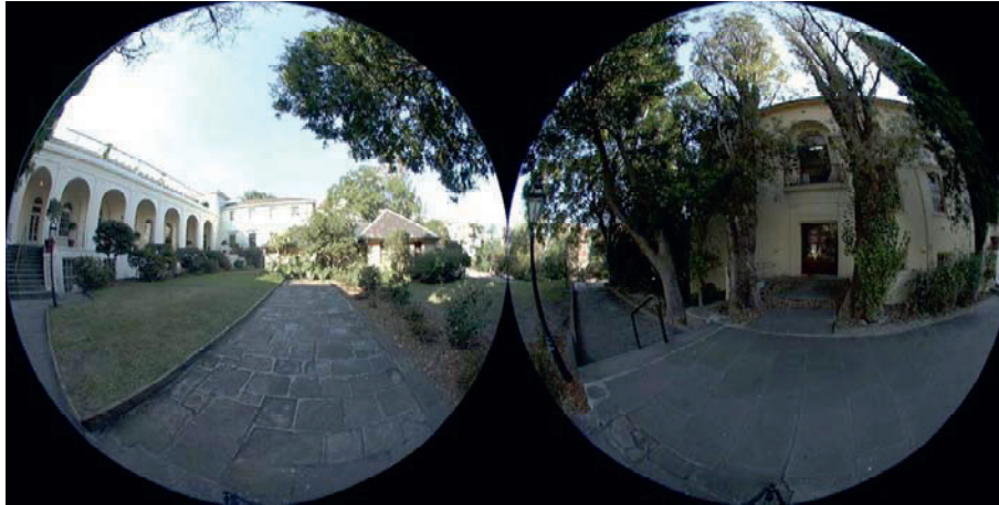
Figure 10: Fish-eye imagery (calibrated luminance map) for point 'a' and used to project for viewpoint specific simulation onto the local and global zones in the VE.
