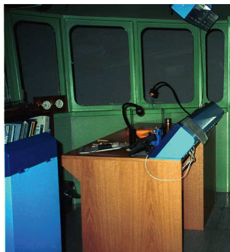
Figure 2. This is a view of the interior of a smaller physical simulator located at DMI. The control panel is an accurate recreation of the instruments on a real ship's bridge. The presence of books and charts is authentic. The 'greyed-out' panels are 'windows' out of which can be seen the virtual scene.
